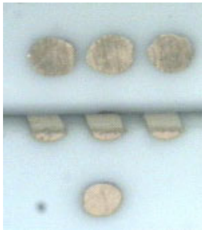
Au Filled Vias in Ceramic Cross Section
